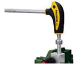
When using the screw socket of the short blade, the longer shank is used as "lever" for extreme torque.
