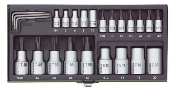
This set contains 1/4" drive (6.3mm) TX sockets in sizes TX8 to TX30 (with frontal hole) and external TX sizes E4 to E8 (all suitable for tightening torques up to 25Nm), 1/2" drive (12.5mm) TX sockets in sizes TX40 - 60 and external TX E10 to E18 (for tightening torques from 25 to 135Nm) and three offset TX spanners - the TX6, 8 and 10. See photo for full contents.
