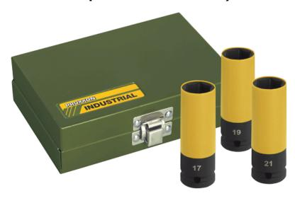
Sockets with plastic cover and plastic stop insert. For use with pneumatic screwdrivers 1/2". Made of high alloy special steel for superior wear resistance and a maximum torque of 500Nm. One piece each 17 - 19 and 21mm in sturdy steel box (powder coated).
