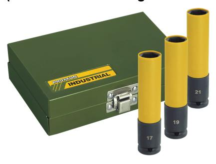
Sockets with plastic cover and plastic stop insert. For use with pneumatic screwdrivers 1/2". Made of high alloy special steel for superior wear resistance and a maximum torque of 500Nm. One piece each 17 - 19 and 21mm in sturdy steel box (powder coated).
