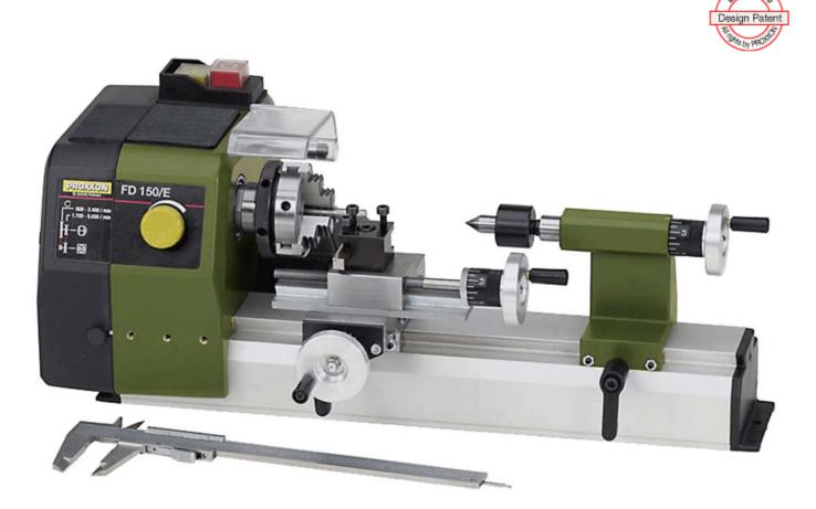
2-stage belt drive and additional electronic control enables spindle speeds up to 5,000rpm. The right cutting speed for even the smallest pieces. For face turning, longitudinal turning, boring, taper turning, slicing and drilling. Complete with 3-jaw chuck and live centre. Centre distance 150mm. Swing 55mm. Height over cross slide 33mm.
