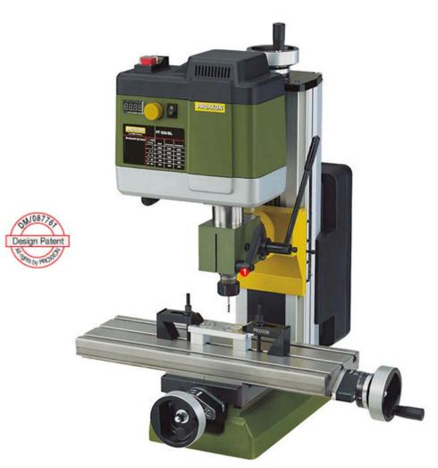
Ouring milling operation the spindle sleeve may be clamped with a T-screw.
