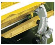
**Table angle adjustment possible from -5° to 50°.** With large dimensioned serrations at 0°, 10°, 20°, 30° and 45°. Additional fine adjustment for precise mitre and angle cuts.
