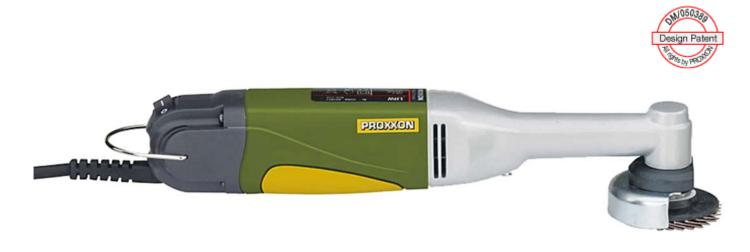
For cutting, rough-machining, grinding and carving wood. Special balanced, powerful, quiet and long-lasting DC motor. Stable head made of glass-fibre reinforced POLYAMIDE. A corundum grinding disc (grit 60), a fan sanding disc (grit 100) and a reinforced cutting disc are included. Safely stored in an attractive and extremely stable case made from polypropylene.
