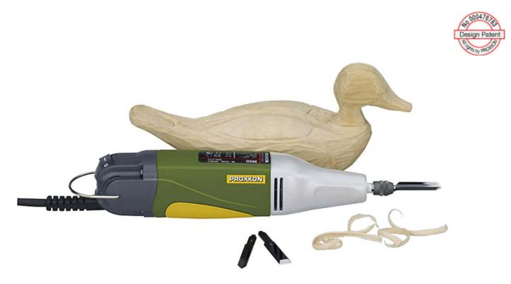
It is also possible to process plaster. Special, balanced, low noise DC motor with extreme high life expectancy. Gear head made of die-cast aluminium. Main housing of glass-fibre reinforced POLYAMIDE. Three high-grade Japanese knife inserts made from bimetal (U-form, V-form and flat blade) are included. In an attractive and extremely stable case made of high-grade polypropylene.
