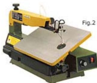
The machine base is made from solid cast iron with rubber feet minimizing vibrations (may also be bolted down). The table is extremely stable with a large work area of 14 5/32" x 10 1/2" (360 x 270mm) and can be tilted 45° for miter cuts (Fig. 2). Vacuum cleaner and dust extractor are side-mounted allowing for a dust-free environment. The machine comes with 5 coarse and 5 fine saw blades each.
