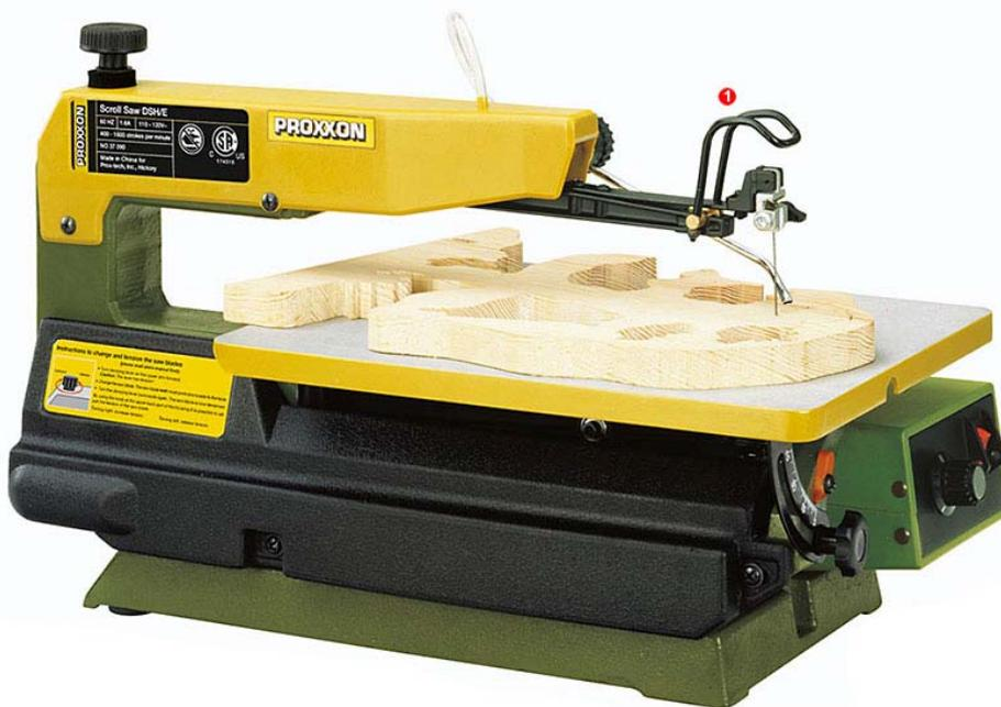
① Practical quick tension release lever (ideal for frequent inside cuts).
