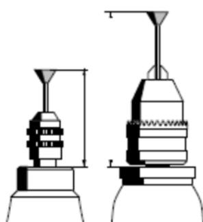
Quality, triple-slit hardened steel collets are ideal for optimum concentricity and tightening force. Furthermore, bits and cutters may be fitted close to the chuck. This is especially important when sanding, routing and milling as side play is minimized.
