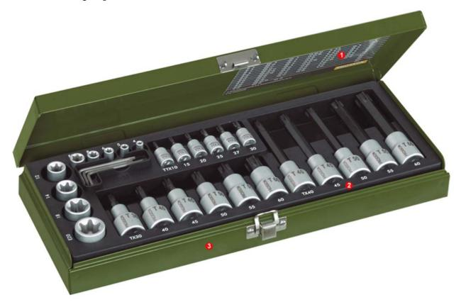
TTX-sockets for 1/4"-square drive (6.3mm). For tightening torques up to 10 Nm: TTX 10 - 30. TX bit sockets in sizes E 4 - 5 - 6 - 8 and 10.
