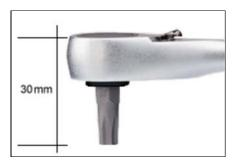
1/4"-MICRO bit ratchet for hexagonal bits. With magnetic insert. Distance between reverse lever and bit end only 30mm. Fine tooth drive: Several of the 72 teeth engage simultaneously for transmitting high torque. Reverse lever for ratcheting direction. Made from CrV steel, double nickel plated with matt chrome plated finish. Grip of oil and acid-resistant TPR (Thermoplastic Rubber). Total length 120mm.
