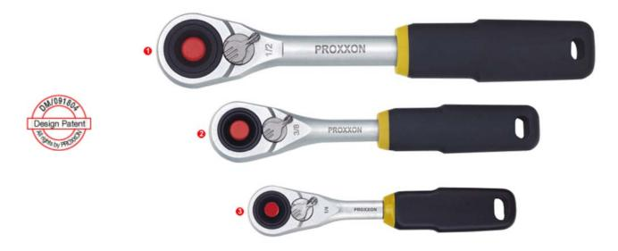
Several of the 72 teeth engage simultaneously transferring extremely high torques. Reverse lever for ratcheting direction. Release mechanism: unlocking the sockets at the push of a button. Forged from CrV-steel, double nickel plated with matt chrome plated finish. Grip of oil- and acid-resistant TPR (Thermoplastic Rubber) with practical hole for hanging up.
