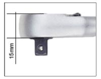
Fine tooth drive: Several of the 72 teeth engage simultaneously transferring extremely high torques. Reverse lever for ratcheting direction. Release mechanism: unlocking the sockets at the push of a button. Forged from CrV-steel, double nickel plated with matt chrome plated finish. Grip of oil- and acid-resistant TPR (Thermoplastic Rubber) with practical hole for hanging up.
