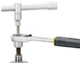
Fitting shock absorbers usually requires a 22mm socket.
