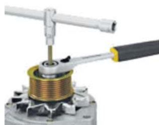
The pulley on an alternator will usually have a 24mm nut.
