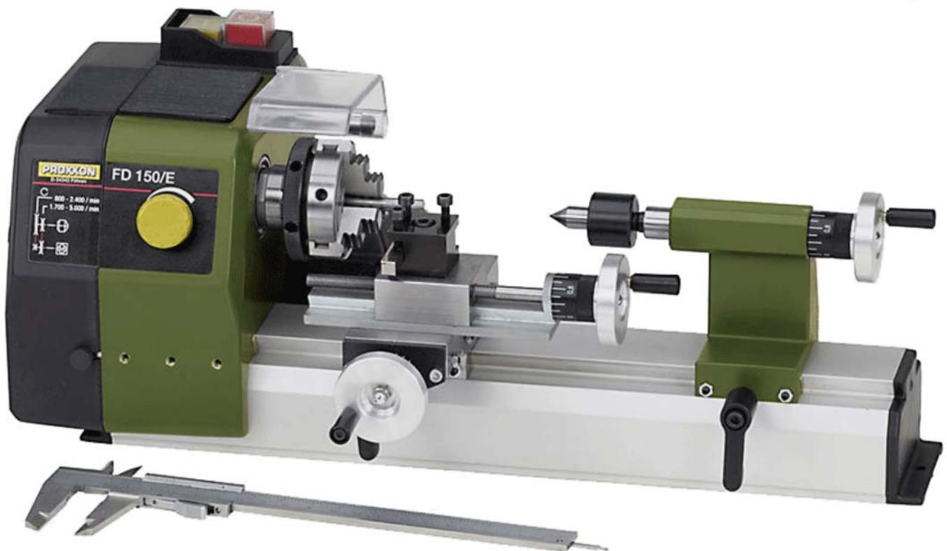
**2-stage belt drive and additional electronic control enables spindle speeds up to 5,000rpm. The right cutting speed for even the smallest pieces. For face turning, longitudinal turning, boring, taper turning, slicing and drilling. Complete with 3-jaw chuck and live centre. Centre distance 150mm. Swing 55mm. Height over cross slide 33mm.**
