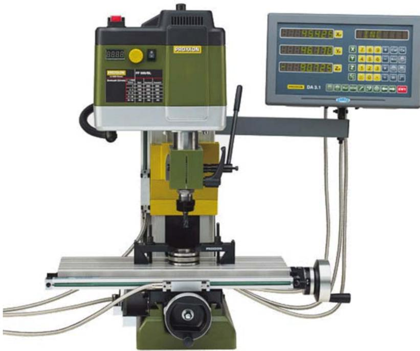
**With large multi-function display, 3 glass rulers (with one sensor each) and fastening elements.**
