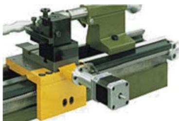
Double roller bearing recirculating ball spindle paired with powerful step motor driven in micro-step guarantee high machining precision and repeat accuracy.
