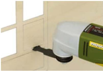
An HSS plunge saw blade (width 14mm) is included.
