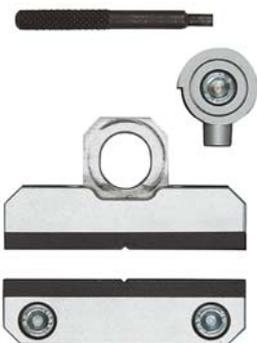
Ideal for series machining and full utilisation of the compound table. Vertical and horizontal prisms for round material. Replaceable clamping jaws. Eccentric stroke 1.5 mm. Jaw width 70 mm. Jaw height 15 mm. Including matching T-nuts and screws.
