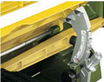
**Table angle adjustment possible from -5° to 50°.** With large dimensioned serrations at 0°, 10°, 20°, 30° and 45°. Additional fine adjustment for precise mitre and angle cuts.
